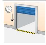
A programmable timer that closes the door after a specified time, counted from either the fully open position and/or from passing through the photocell beam.
