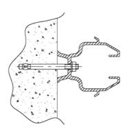
Secure the guide rails with self-threading screws
