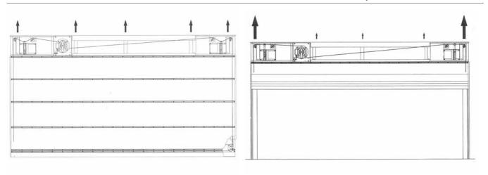
When the door is closed, the total weight is distributed on the fixing points. The distance between fixing points is about 1000 mm. The door leaf itself does not weigh more than 40 to 80 kg per meter width but, in view of the extra load which may result in the event of a collision, the total load of the building should be calculated at 1.5kN/m.
