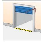
A pull rope switch next to the door opening can be operated from e.g. a forklift truck. Pulling the rope opens a closed door or closes an open door.
