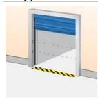
Two sets of photocell transmitters with reflectors and receivers are installed in the door opening. If one or both photocell beams are interrupted during closing, the door will stop in less than 30mm and reverse to the fully open position.
