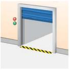
One or two sets of green and red lights indicating that the door is open or closed; continuous green light when the door is open, continuous red light when the door is closed, optionally flashing light when the door is moving or not fully open.
