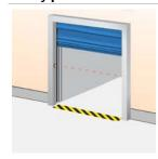
A set of a photocell transmitter with reflector or receiver is installed in the door opening. If the photocell beam is interrupted during closing, the door will stop in less than 30mm and reverse to the fully open position. Installed in the door opening.
