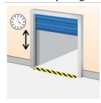
A programmable timer that closes the door after a specified time, counted from either the fully open position and/or from passing the photocell beam. A sensor, e.g. a magnetic loop or radar, is used for automatic opening.
