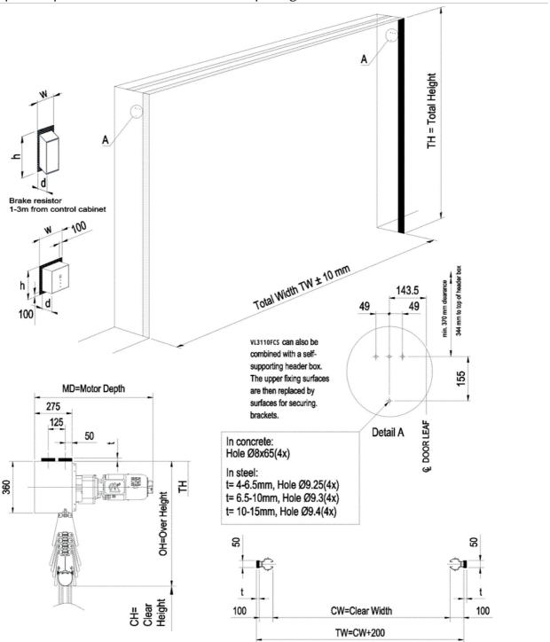
The VL3110FCS vertical lifting fabric door can also be provided with a self-supporting header box. The upper fixing surfaces are then replaced by surfaces for securing brackets.
