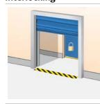
Developed for climate control or safety; if door A is open, door B cannot be opened. If door B is open; door A cannot be opened.
