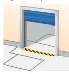
A sensor in the floor detects a metal object (usually forklift trucks, pallet trucks) and opens the door automatically. This is an ideal solution for frequent vehicle traffic
