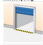
When it is unnecessary or undesirable to fully open a door, an absolute encoder is used to configure a reduced opening position.
